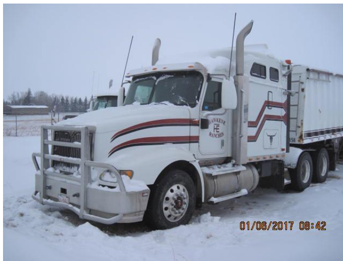
9159D-1-2006 IHC Hiway tractor, unibody bunk, Cummins ISX, 525 HP, 18spd, air ride, Aluminum Budds, wet kit, air slide 5 th wheel, 40,000lb rear axle (3.90 ratio), 3 way lockers, electric brake control, goose neck ball, bush bumper, beacons, 1, 107,872 Km, 69,074 km on complete engine re-build. VIN: 2HSCNAPRX6C319715
